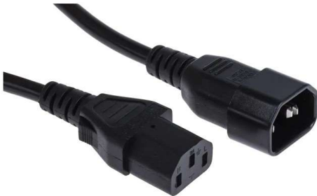
FCR72039 - IEC C13 PLUG TO IEC C14 PLUG 2m PVC Cable H05VV-F 3x1.0mm 2
